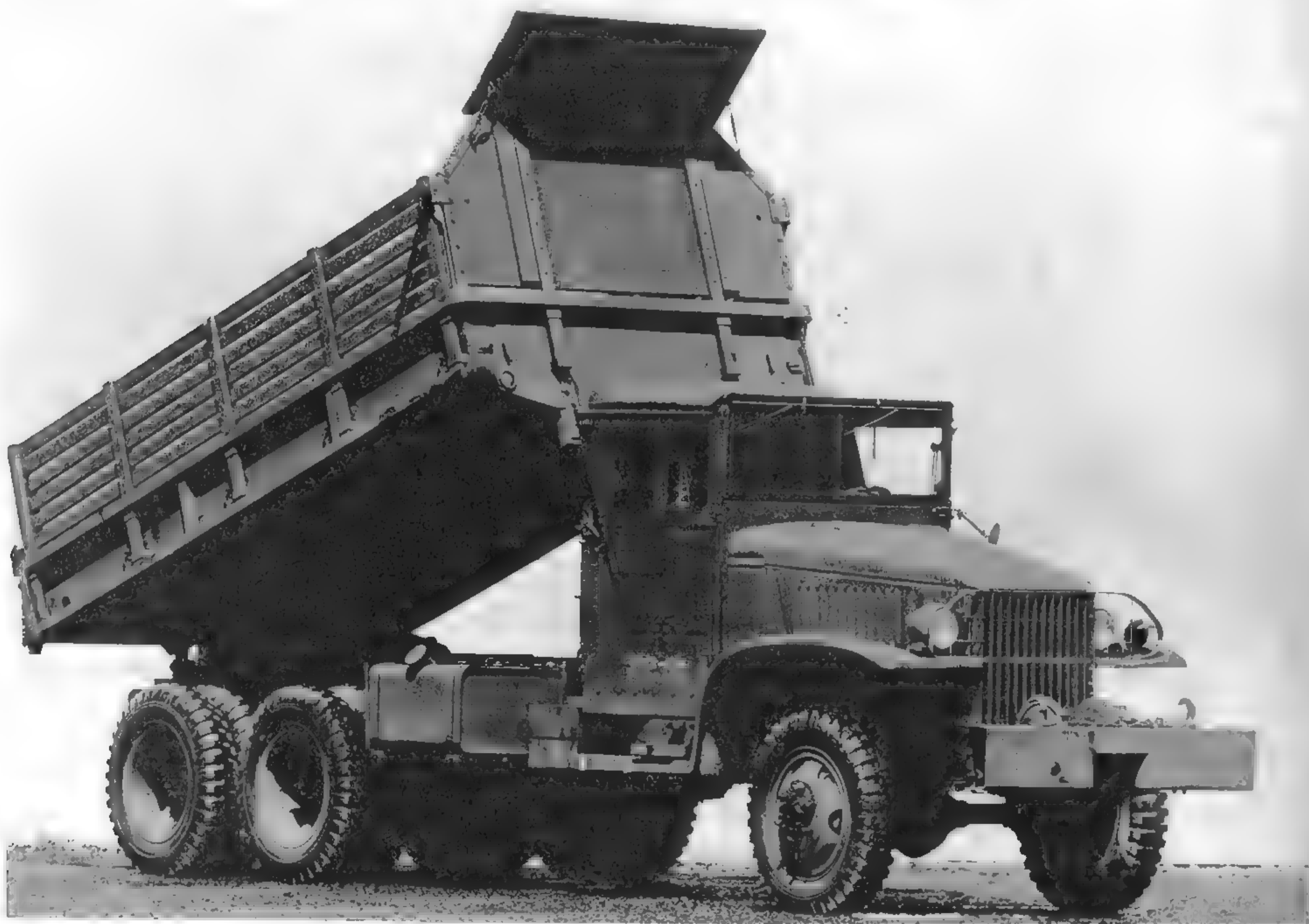
This typical CCKW tipper was photographed in 1944 in South Bend, Indiana. Notice the damage to the lower front corner of the bed of this otherwise factory-fresh truck. (U.S. Army photo)
